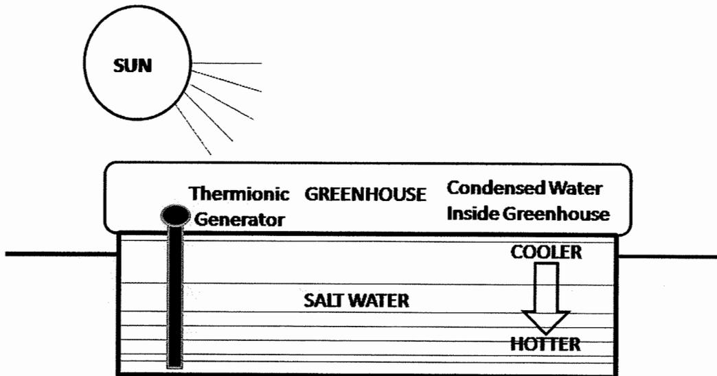
**SOLAR PONDS:** These can make fresh water from condensation in the greenhouse, however, the salt water inside the greenhouses uses the saline difference to create electricity via a heat transfer fluid, or heat engine. The salt water is hotter at bottom, than the salt water at top of the pond. The temperature difference can drive a low temperature working fluid to drive a small turbine.
